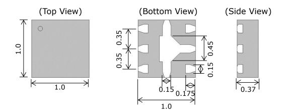
6GHz Middle Power SPDT Switch for Wireless LAN
