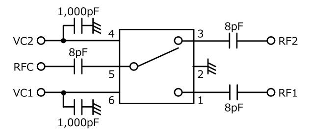
The application circuits and their parameters are for reference only and are not intended for use in actual design-ins. This device is used it is necessary to use DC Block Capacitance.
